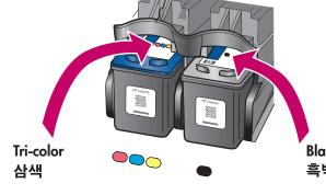
Hold the color print cartridge with the large HP label and the raised markings on top. Slide the cartridge at a slight angle into the left side of the print carriage.
